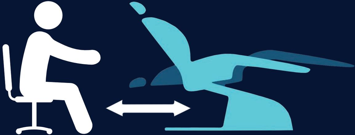
Engle is the only company that makes the "fully programmable 10.25" forward/backward hydraulic Traverse Chair™. The traverse feature allows dentists to position themselves behind the patient comfortably without sacrificing space. Since the seat moves forward as the back of the chair reclines, you can stay put and let the patient come to you.
